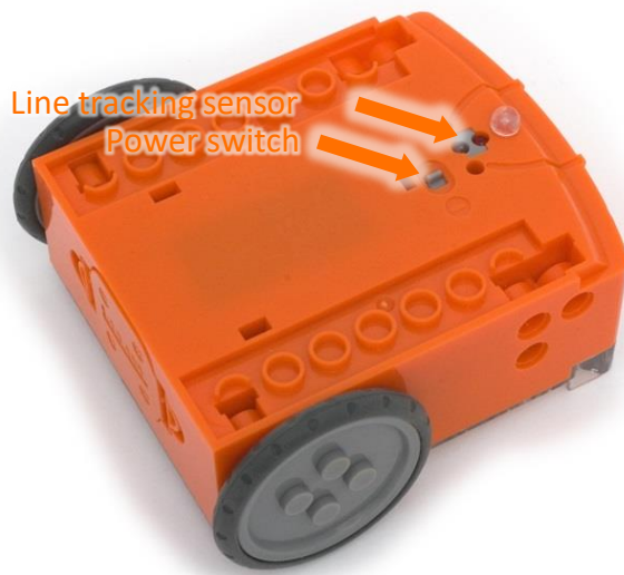
Location of Edison's power switch and line tracking sensor.
